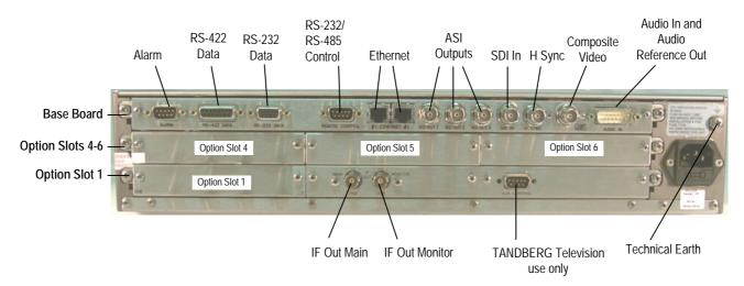
Figure 2.5: E5740-IF (2U) Rear Panel Component Parts and Connectors
